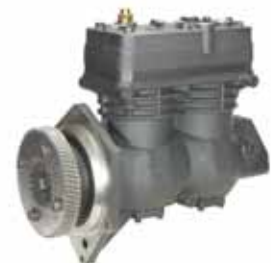
BA-922® Compressor 31.6 CFM AT 1250 RPM
